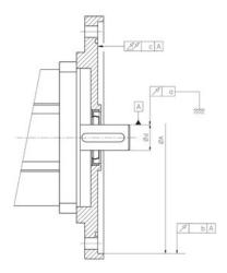
Fig. 5.1.5: Required tolerances of the T series a) valid for TS 70, TS 110, TS 140, TS 170, TS 200 b) valid for TS TS 80, TS 240, TS 300
