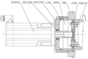
Fig. 5.2.1a: Direct connection of the reduction gear shaft with the motor shaft
