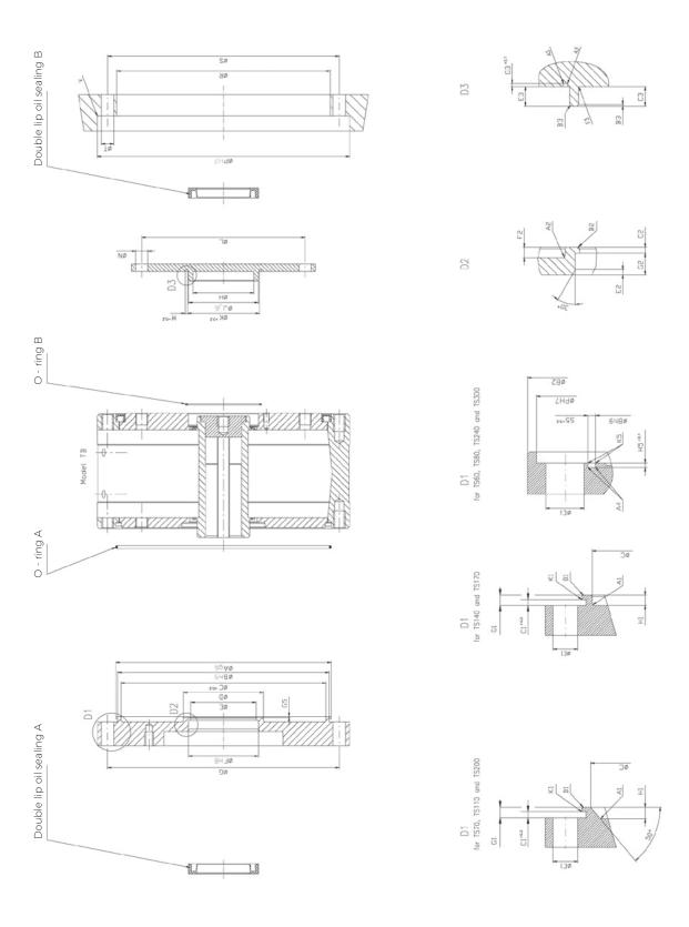
Fig. 5.1.4a: Dimensions of input and output flanges of the TwinSpin $^\circ$  T series reduction gear
