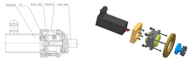
Fig. 5.4.1a: Shaft connection with a keyway
