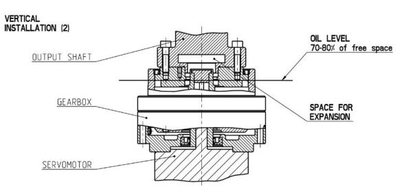
Fig. 5.5a: Lubricant levels in horizontal and vertical positions
