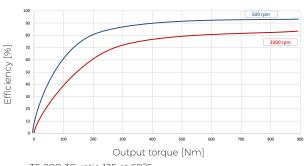
TS 200-TC, ratio 125 at 60°C H = 0.71 arcmin LM = 0.5 arcmin Max. speed = 3 000 rpm
