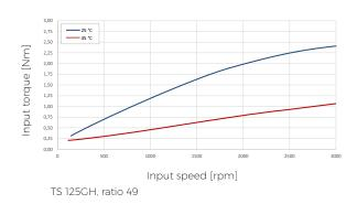
Fig. 3.16: No-load running torque charts
