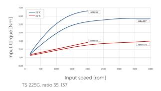
Fig. 3.15: No-load running torque charts
