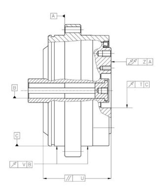
Fig. 5.2.4b: Tolerances of circumferential and face runout in the case of direct connection of TwinSpin $^{\circ}$  high precision reduction gears with a servomotor according to DIN 42955 R
