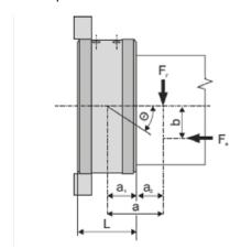
Fig. 3.6a: Load and moment on the T, E, H, M series output flange
