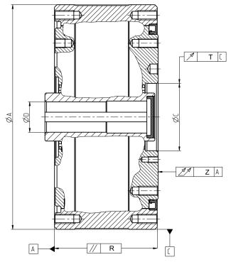
Fig. 5.1.6a: Tolerances of circumferential and face runout for direct connection of TwinSpin® high precision reduction gears with a servomotor in accordance with DIN 42955 R
