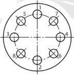
Fig. 12.2: Tighten the screws along the perimeter of a circle in a cross-like manner
