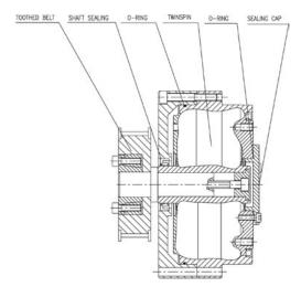
Note: The sealing cap is used only with reduction gears TS 110, TS 140, TS 220 Fig. 5.2.1c: Connection of the reduction gear with a toothed pulley
