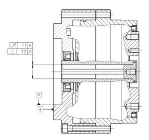
Fig. 5.2.4a: Geometric deviations for the connection of the E series TwinSpin® high precision reduction gear flange with a motor or of the TwinSpin® E series reduction gear
