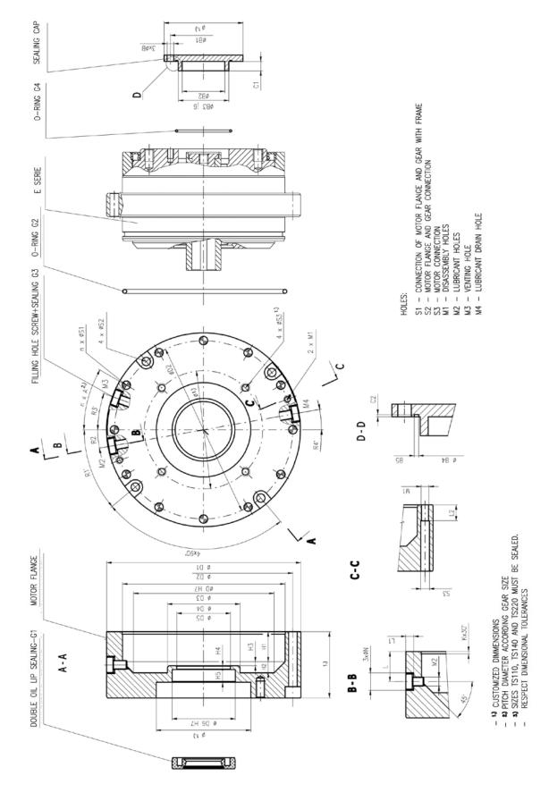
Dimensions and tolerances of the E series connecting components
