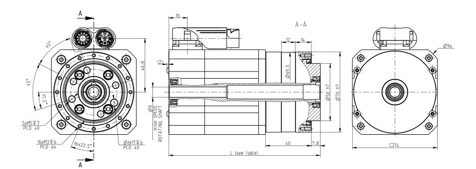
Hollowshaft rotates at motor speed
