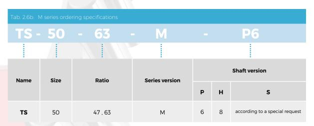
Note: An example of an ordering code of a modified TwinSpin® reduction gear with with a motor flange:
