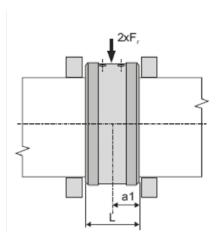
Fig. 3.6b: Load and moment on the T, E, H, M series output flange
