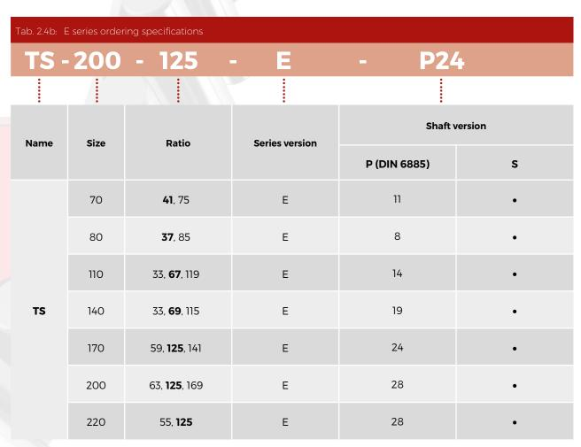
Note: An example of an ordering code of a modified TwinSpin® T series reduction gear with a motor flange: TS200 - 125 -TC- P24 - M235 - P231. The markings M235 and P231 for a specific modification are defined by the manufacturer.
