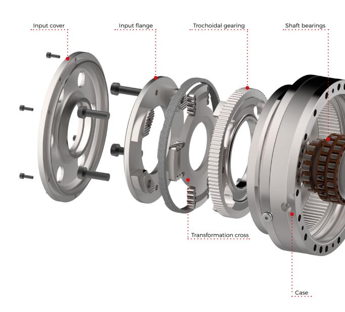
Fig. 1.a: TwinSpin® reduction gears components
