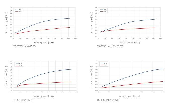
Fig. 3.15: No-load running torque charts
