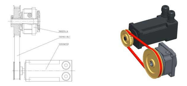
Fig. 5.4.1d: Example of the use of the hollow-shaft version of the reduction gear, driven through a toothed belt
