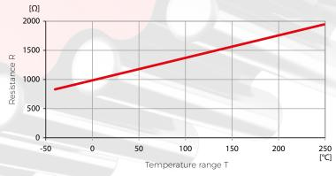
Fig. 9.10: Resistance / Temperature PT 1000
