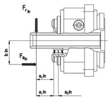
Fig. 3.12a: Radial load of the T, E, H series input shaft
