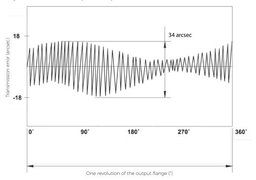
Fig. 3.9: Angular transmission error measurement
