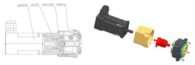
Fig. 5.4.1b: Shaft connection with a flexible coupling
