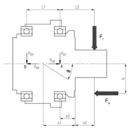
Fig. 3.5.1: Loading of the M series reduction gear and the angle of tilt
