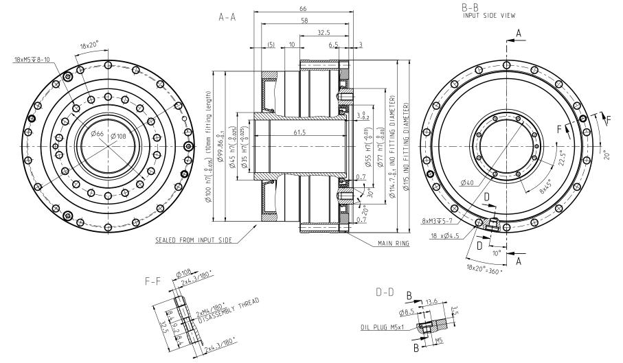
1. Main ring must be fixed in operation with 18pcs of screw M3, st 12.9, tilghtening torque  $5\ Nm$
