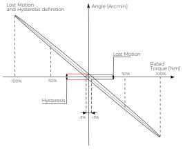
Fig. 3.7a: T, E, H, M series hysteresis curve and the definition of stiffness
