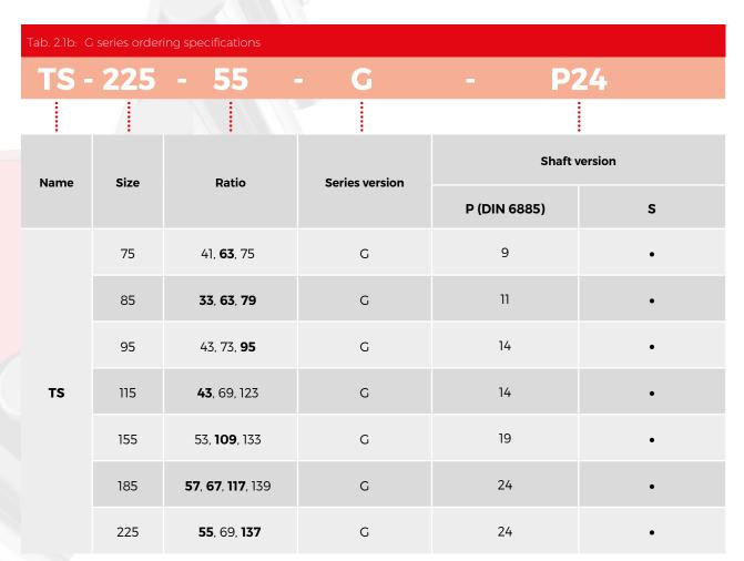
Note: An example of an ordering code of a modified TwinSpin® G series reduction gear with a motor flange: TS225 - 55 -G- P24 - M235 - P231. The markings M235 and P231 for a specific modification are defined by the manufacturer.
