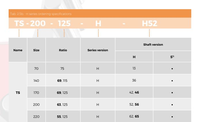
Note: An example of an ordering code of a modified H series TwinSpin® reduction gear with a motor flange: TS200 - 125 - H- H56 - M235 - P231. The markings M235 and P231 for a specific modification are defined by the manufacturer. 1) On request
