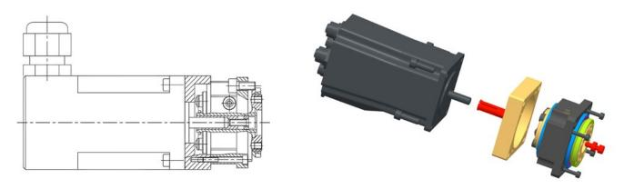
Fig. 5.4.1c: Shaft connection with a collet
