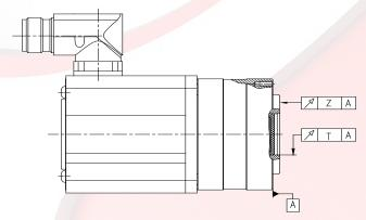
Fig. 12.1: Axial and radial runout to base A
